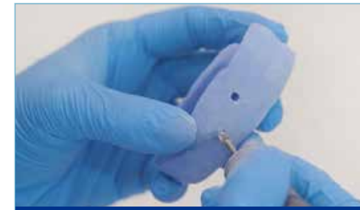
⑤ Drill two venting channels
